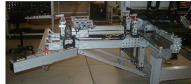
ZT and ZF for workplace for installing plastic parts on fluid containers.
