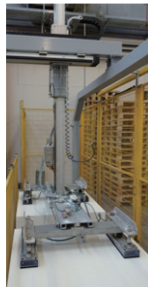
ZSS for pick and place of large foam components (manufacturing of rotor blades for wind turbines).
