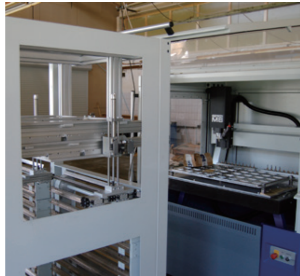
Supply unit for workpieces to be machined, clamped in machining fixture.
